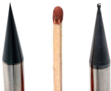
Comparison of micro-endmill (0.2mm) and normal endmill (1.0mm)
