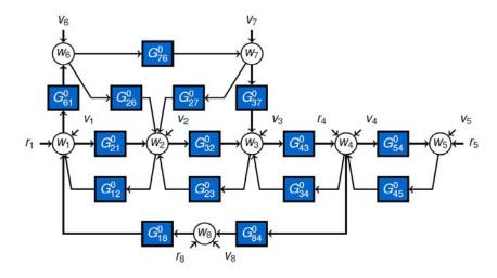
r<sub>i</sub> external excitationv<sub>i</sub> process noisew<sub>i</sub> node signal
