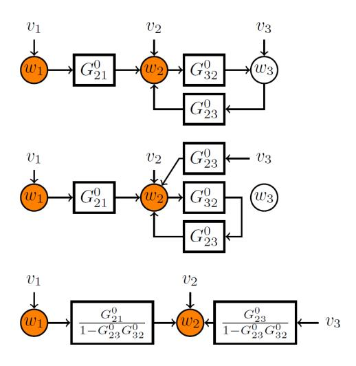
Removing path through  $w_3$  called *lifting a path*.
