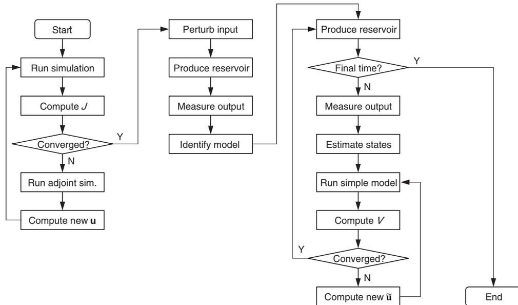
**Fig. 2—Flow chart of the two-level strategy. The left column represents life-cycle optimization by use of a large-scale reservoir-simulation model (performed only once in our example). The second column represents identification of a data-driven model (also performed only once in our example). The third column represents computation of tracking control input by use of the identified model.**
