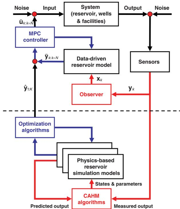
**Fig. 8—Two-level strategy to combine closed-loop reservoir management based on multiple models (bottom part of the figure) with tracking control of production (top part of the figure).**
