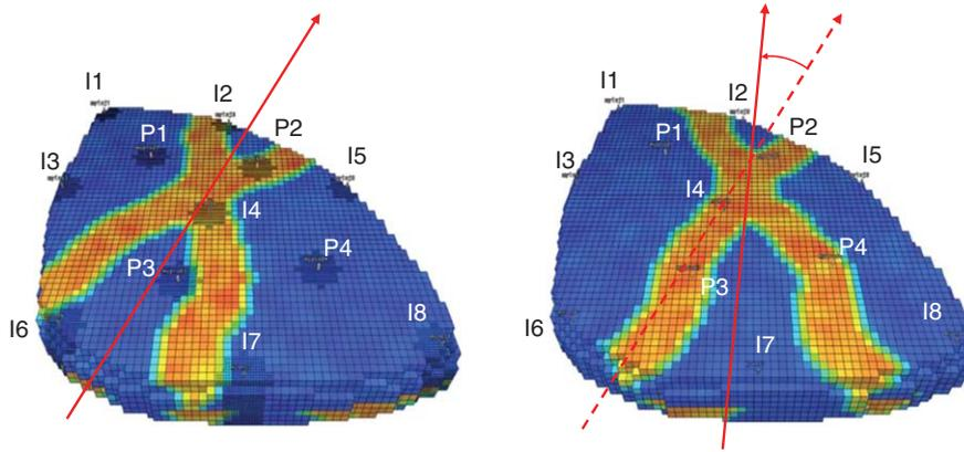
**Fig. 3—3D reservoir model (left), used as synthetic “truth,” with eight injection wells and four production wells. Its geological structure involves a network of meandering channels of high permeability. The model to the right is used for life-cycle optimization and differs from the model to the left in the direction of the channels, the absence of grid refinement, and the larger timestep size of 30 days.**
