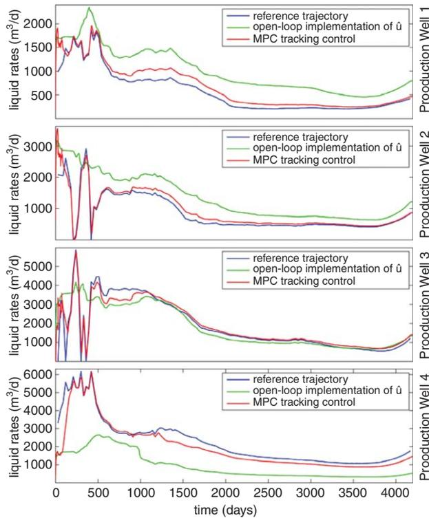
**Fig. 7—Reference and output trajectories for the open-loop application and the tracked case for each of the four production wells over the life of the field.**
