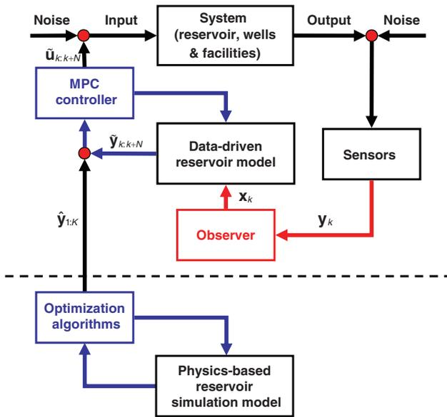
**Fig. 1—Two-level strategy to combine life-cycle optimization (bottom part of the figure) with MPC tracking of production (top part of the figure).**
