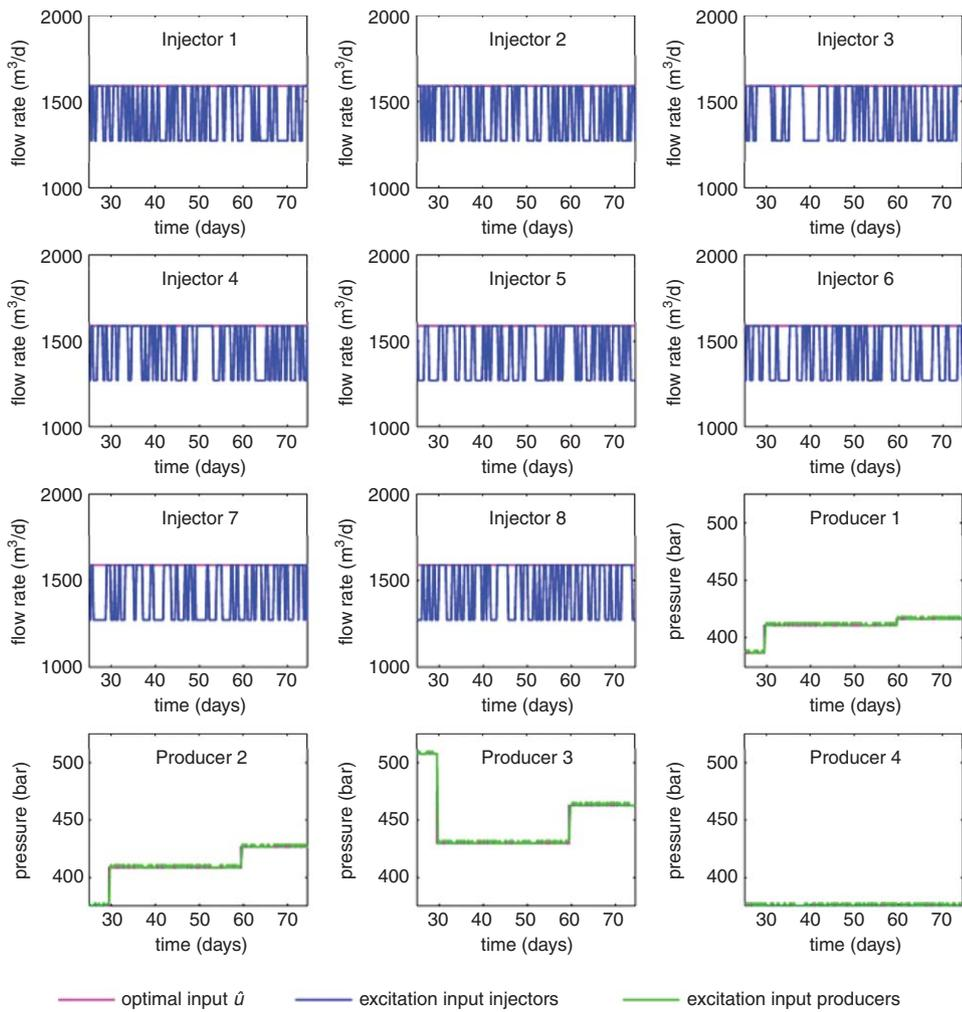
Fig. 4—Excitation signal for the identification experiment along with optimal inputs  $\hat{u}$  for each input.
