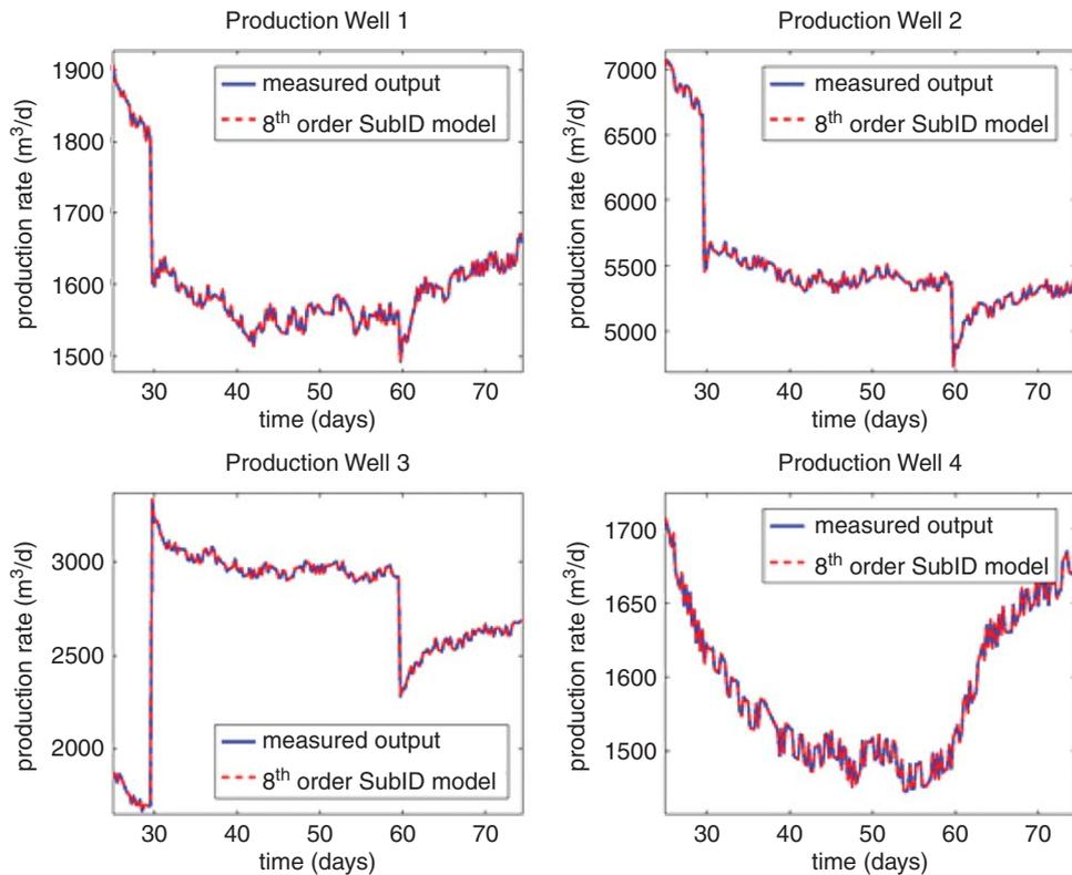
Fig. 5—Model fit of the eighth-order SubID model with respect to the measured output data.
