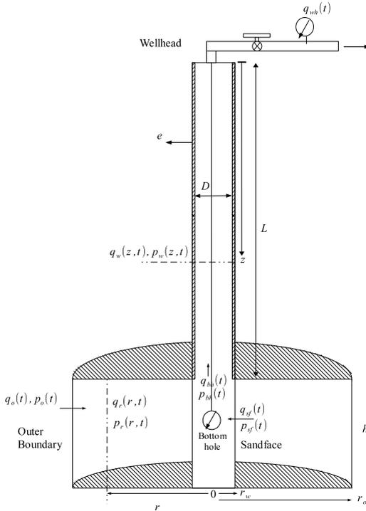
Figure 8.1: A cylindrical homogeneous reservoir with a vertical well. This figure was created by Mehdi Mansoori (Mansoori et al., 2014)
