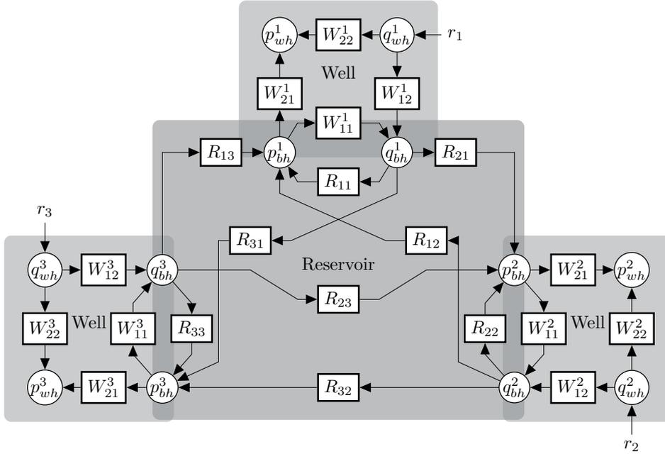
Figure 1.4: Model of the three wells and reservoir shown in Figure 1.3 using transfer functions. The variables  $p_{bh}^i$  and  $p_{wh}^i$  denote bottomhole and wellhead pressures of well  $i$  respectively;  $q_{bh}^i$  and  $q_{wh}^i$  denote bottomhole and wellhead flow rates respectively;  $r_i$  denotes the flowrate that can be externally controlled using a valve. The transfer functions  $W_{ji}$  denote the dynamics of wellbore  $k$ , and  $R_{ji}$  denote the dynamics of the reservoir.
