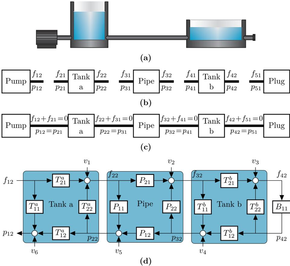
Figure 2.5: Simple hydraulic system.
