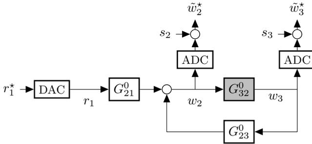
Figure 7.3: Closed loop data generating system considered in Example 7.7
