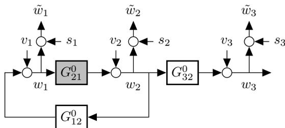
Figure 6.4: Data generating system considered in Example 6.22
