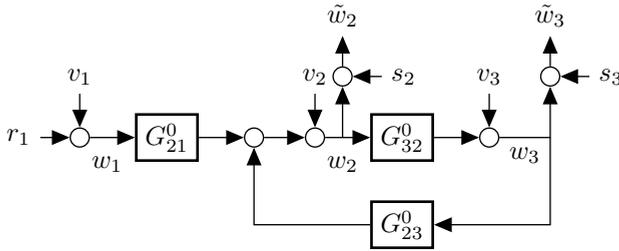
Figure 3.5: Closed-Loop data generating system with sensor noise.
