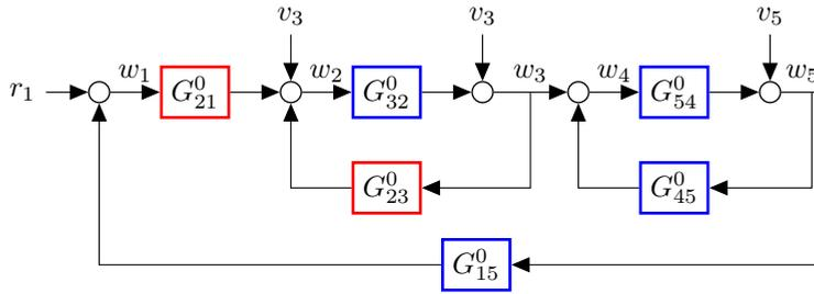
Figure 4.2: Dynamic network with 5 internal variables, of which 2 (red-colored) transfer functions  $G_{21}^0$  and  $G_{23}^0$  can be consistently identified with the direct method using a MISO predictor. The blue-colored transfer functions can be identified with SISO predictors.
