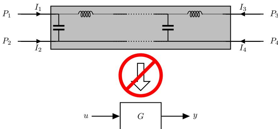
Figure 1.7: A lossless transmission line.  $I$ 's denote currents, and  $P$ 's denote voltage potentials and a transfer function representation of the transmission line.
