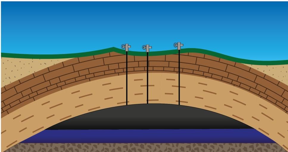
Figure 1.3: Diagram of three wells. The brown layers denote layers of rock, the black layer denotes a permeable layer where oil has gathered, and the blue layer denotes a water layer. The rock formation shown is an *anticline* formation. Reservoirs often are found in this type of formation (Dake, 1983).
