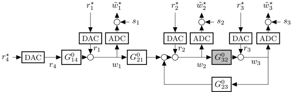
Figure 7.1: Closed loop data generating system with no process noise and continuous-time external variables that are constructed from discrete-time external variables (using DACs).
