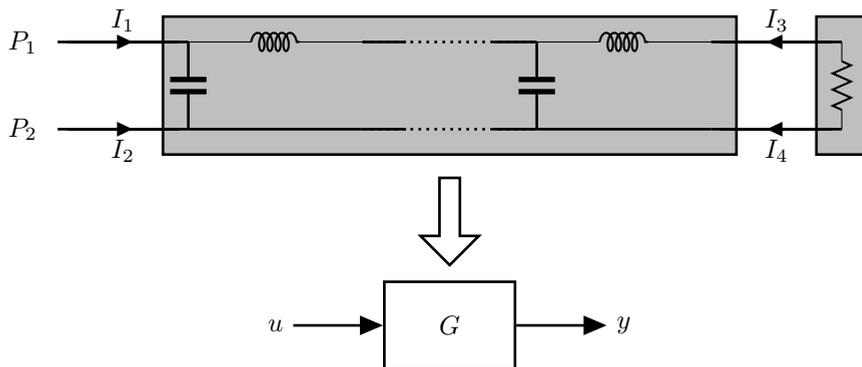
Figure 1.8: A lossless transmission line with a termination.  $I$ 's denote currents, and  $P$ 's denote voltage potentials and a transfer function representation of the transmission line.
