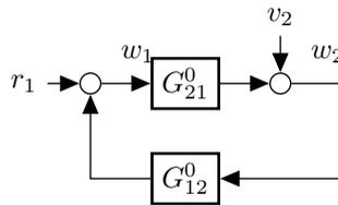
Figure 3.1: A typical closed loop system considered in the identification literature.
