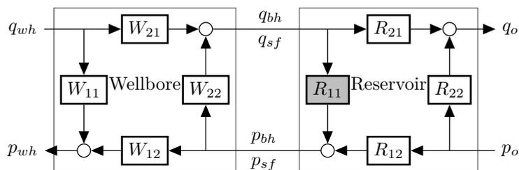
Figure 8.2: Bilaterally coupled reservoir and well bore model.
