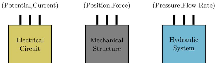
Figure 2.4: Examples of systems with terminals (Willems, 2007). The terminals are shown in thick lines, and the variables living on those terminals are indicated in brackets.
