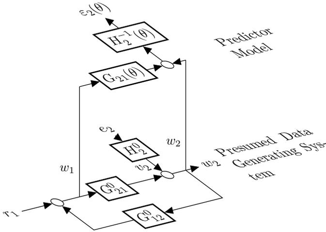
Figure 3.3: Closed-loop identification setup.
