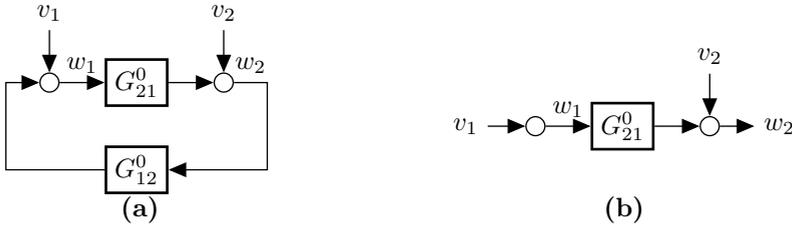
Figure 1.10: Open and Closed-loop data generating systems considered as candidate data generating systems considered in Caines & Chan (1975); Caines (1976); Anderson & Gevers (1982); Gevers & Anderson (1981, 1982). The  $v$ 's denote stochastic processes with rational power spectral density.
