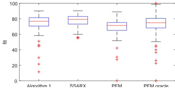
Fig. 3. Fit of  $G_{12}$  for 100 randomly generated systems and data sets for: Algorithm 1, SSARX, PEM with standard initialization, PEM initialized by true system.
