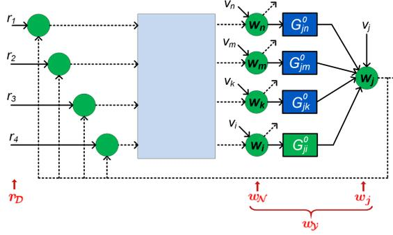
Figure 2: Predictor model for the indirect method.
