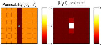
Fig. 4. Permeability distribution containing a streak with lower permeability values (left) and corresponding dominant spatial patterns in parameter space (right).
