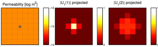
Fig. 2. Top view of a homogeneous permeability distribution with well location indicated by a grey dot (left) and corresponding dominant spatial patterns in parameter space (middle and right).
