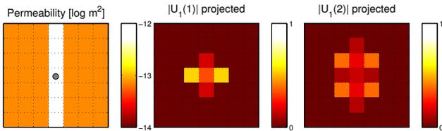
Fig. 3. Permeability distribution containing a streak with higher permeability values (left) and corresponding dominant spatial patterns in parameter space (middle and right).
