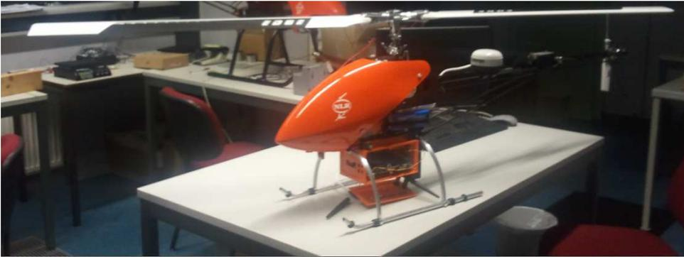
Figure 1.16: NLR's mini-UAV project (2012-2014) based on a modified Align T-REX helicopter.
