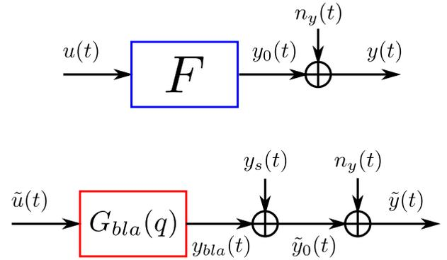
Fig. 2. A dynamic nonlinear system ( $F$ ) with zero-mean (colored) additive noise  $n_y(t)$  at the output only (top) is represented as the Best Linear Approximation of the system behavior  $G_{bla}(q)$  and a stochastic nonlinear distortion source  $y_s(t)$  (bottom).
