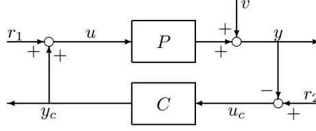
Fig. 1. Feedback connection structure  $\mathcal{T}(P, C)$ .
