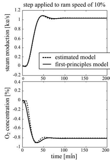
Fig. 3: Responses of steam and O<sub>2</sub> to step on ram speed
