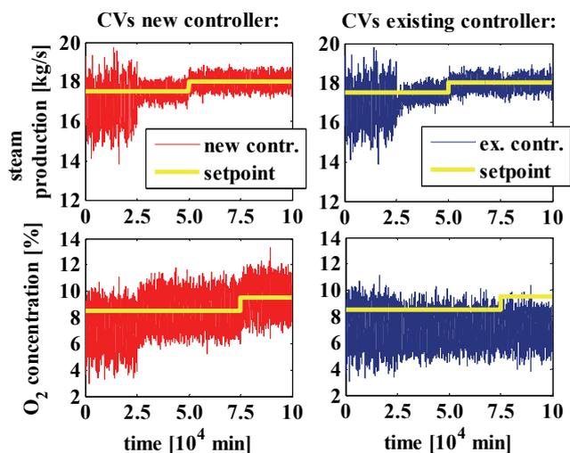
Fig. 9: New versus existing controller
