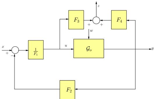
Fig. 2. Generalized Virtual Closed Loop.
