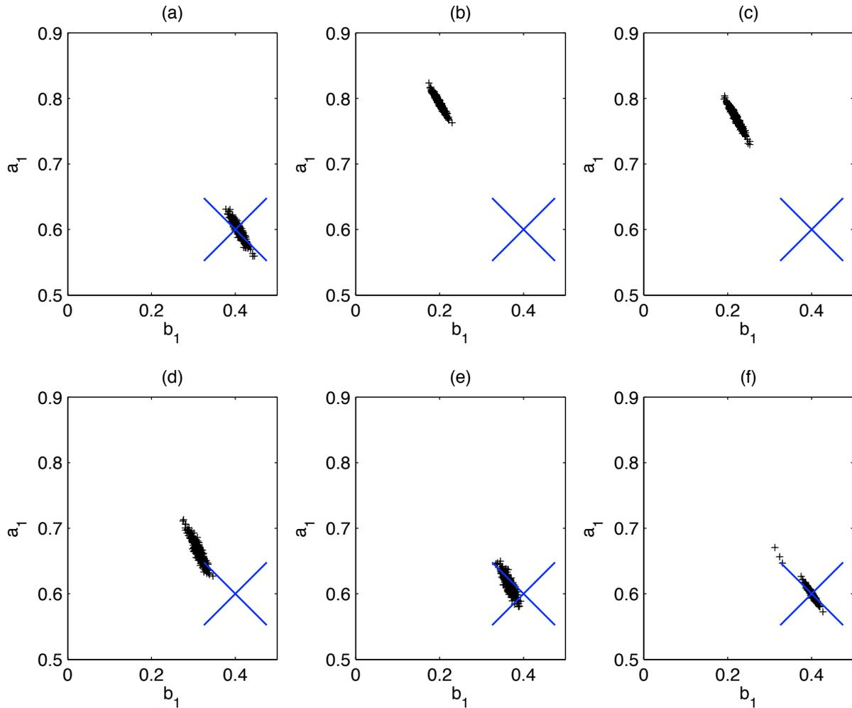
Fig. 6. Results for 300 Monte-Carlo experiments. True value (big-blue-cross). (a) VCL with an output error model ( $K = 1$ ), (b) Direct identification with an output error model ( $H = 1$ ), (c) Direct identification using a noise transfer model with  $n = 1$ , (d) Direct identification using a noise transfer model with  $n = 2$ , (e) Direct identification using a noise transfer model with  $n = 3$ , (f) Direct identification using a noise transfer model with  $n = 4$ .
