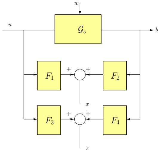
Fig. 1. Signal Generation in the Virtual Closed Loop Method.
