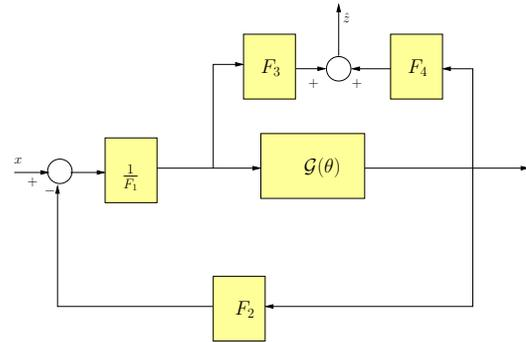
Fig. 3. Predictor Model for the Generalized Virtual Closed Loop.
